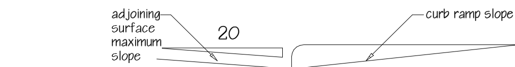
Fig. 406.2 Counter Slope of Surfaces Adjacent to Curb Ramps
